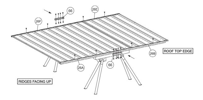
Enhance the structural strength by applying part 66 (channel connector). Note that screws are applied to both sides of the connectors.
