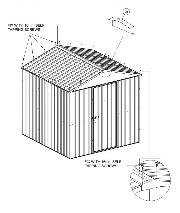
Now fit the bolt down kit as per the diagram below. Strengthen your mid wall brace by applying part 72 (mid wall brace bracket) to each corner if necessary.
